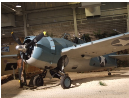
The F4F Wildcat on display in the museum is a dash-3 variant, with four .50 caliber guns and non-folding wings.
